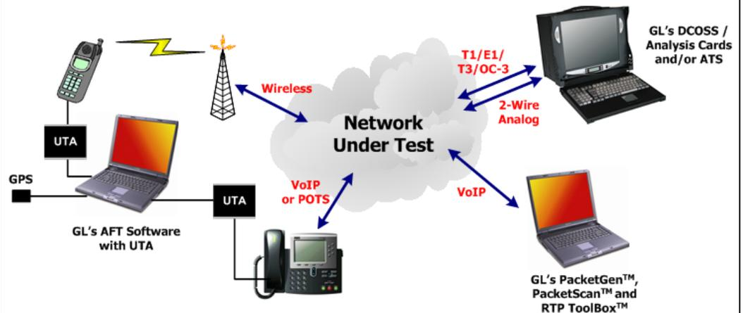
Providing clear, uninterrupted voice is critical in Network and Echo Cancellation development. GL's Voice Quality Testing (VQT), accessed through an easy to use GUI interface, provides the voice quality measurement and analysis tools for all types of networks carrying voice traffic. Typical network applications include VoIP systems, PSTN, ATM networks, Frame Relay, and Wireless Networks.
